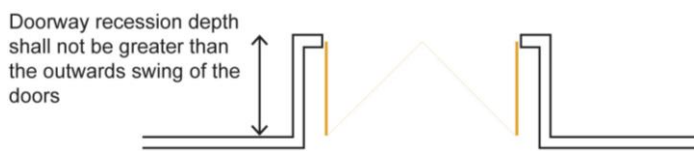
Figure 29. Doorway Recession Regulations
