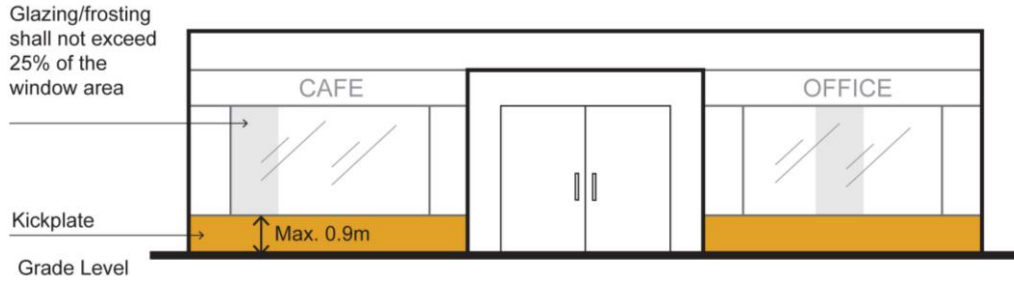
Figure 28. Building Facades Regulations
